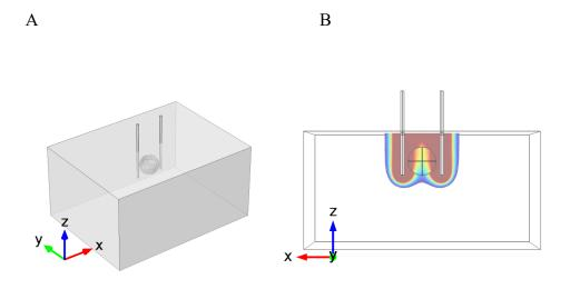
**Figure 1:** (A) Simple 3D model of tumor and needle electrodes in healthy tissue; (B) electric field over reversible threshold inside the healthy tissue and the tumor.
